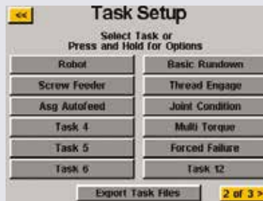
The tasks can be downloaded, allowing fast and simple backup of the machine with a simple key press (Export Task Files)
